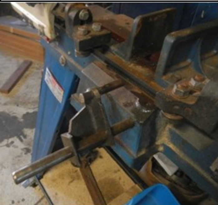
Photo 4 – new feed stop installed – note result of oil spill in background.
